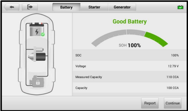
Figure 10-7 Battery Test Results Screen
